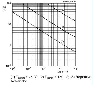
Fig. 2. Avalanche rating; avalanche current as a function of avalanche time
